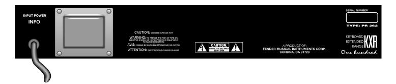
NOTE: DO NOT BLOCK THE AIR FLOW TO THE REAR PANEL; FOR EXAMPLE, BY BACKING THE AMPLIFIER UP AGAINST A WALL. The rear panel is used to keep the output devices from getting too hot.
